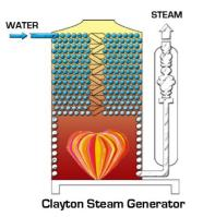
This is possible by pumping water through the inside of a small diameter heated coiled tube so that cold water goes in one end and high pressure steam comes out the other. The Clayton Steam Generator is a unique design that does just that. Instead of the familiar steam train image of a boiler we now have a compact steam making machine with staggering advantages for the world we live in today.
