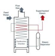
where it is pre-heated as it spirals downwards and fed to the lower section from where it passes to the high efficiency steam separator. Dry steam from the separator is then directed to the integral superheating coil section where the desired steam temperature is produced.
